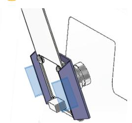
Place cover over camera with the camera lens through the center hole. Secure with tape.
